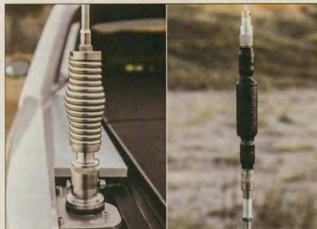
Figure 3 — Close-ups of (left) optional base spring, and (right) the completed loading coil.
