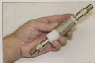
Figure 1 — Partially completed coil assembly attaches on top of the mast and supports the whip assembly.
